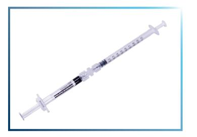
Figure 1. Attach the connector to the luer on the glass syringe and connect the tuberculin syringe to the other end of the connector
