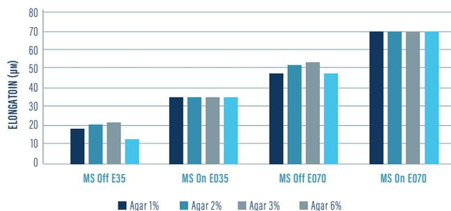
Figure 2. Actual tip elongation in sculpt phase, with feedback control on and off when nominal elongation was programmed by the surgeon at 35 µm (E35) and 70 µm (E70). The dark blue, light blue, gray, and teal bars indicate increasing agar gel percentage, mimicking the increasing hardness of the cataract material.
