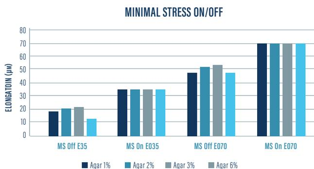
Figure 2. Actual tip elongation in sculpt phase, with feedback control on and off when nominal elongation was programmed by the surgeon at 35 µm (E35) and 70 µm (E70). The dark blue, light blue, gray, and teal bars indicate increasing agar gel percentage, mimicking the increasing hardness of the cataract material.
