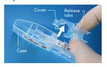
Press the release tabs, lift up and remove the cover from the case.
